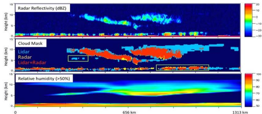
CloudSat radar and CALIPSO lidar can be used to accurately determine the heights of multilayered clouds, and provide *a priori* training for GOES-16.
