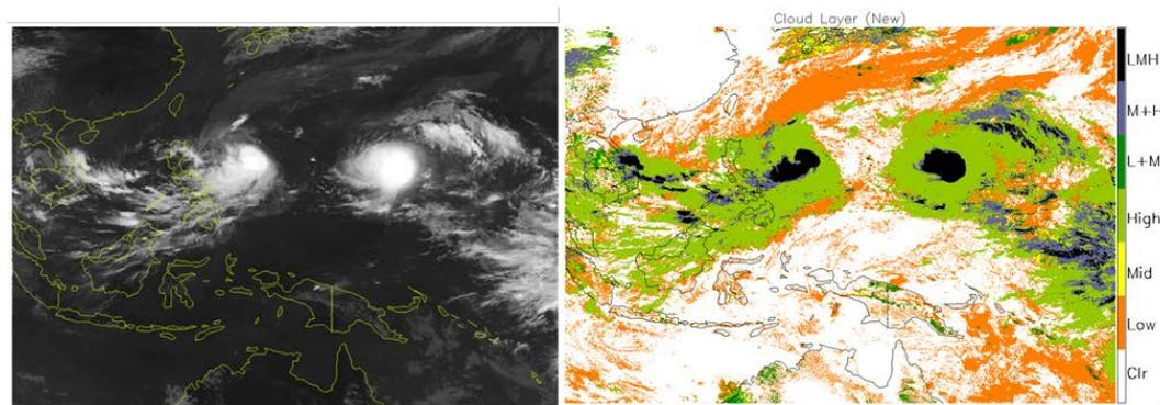
Combined cloud layer flags (L=low, M=mid, H=high) (right panel) produced by the CIRA cloud geometric thickness algorithm (right) applied to Himawari-8 AH1; 11  $\mu\text{m}$  IR image (left).
